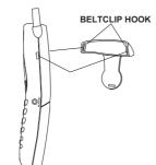
With the back of the HANDSET facing up, insert one side of the BELT CLIP HOOK into the matching slot at the top side of the HANDSET. Press down on the opposite side of the BELT CLIP until the other hook locks Into the slot on the side of the HANDSET.
